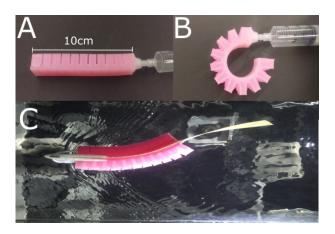
Fig. 1. A) An uninflated pneunet connected to a syringe. B) A fully inflated pneunet. C) As seen from below, a pneufish operating in water. The cuff (left end of the pneufish) connects to a dorsally-located vertical rod housing the force and torque transducer. Image C adapted from [8].
