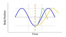
Fig. 2. Predicted results of Aim 1. Body stiffness is modulated at the time corresponding to the orange dotted line. If stiffness is increased (green), the cycle will shorten. If stiffness is decreased (yellow), the cycle will lengthen.
